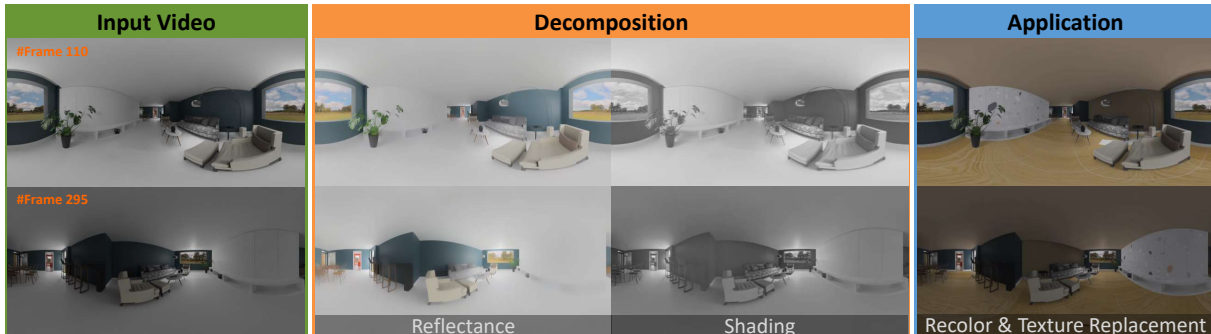
Figure 1: An input omnidirectional video (left) is decomposed into its reflectance and shading components (middle) by the proposed method. The decomposition results can be further used for video manipulation applications (right).
