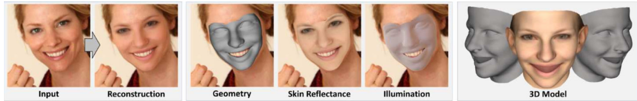
Fig. 4 Model-based neural network for unsupervised monocular reconstruction. The proposed face autoencoder enables unsupervised end-to-end learning of semantic parameters including geometry, illumination, expression, etc. Reproduced with permission from Ref. [64], © Institute of Electrical and Electronics Engineers 2017.
